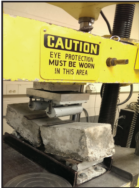
Figure 1. Flexure test of PMC beam
